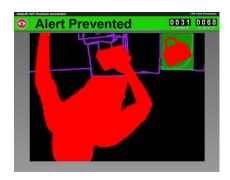
NCR's technology flags scan-avoided merchandise and unscanned merchandise left in the shopping cart – and sends a real-time alert to the attendant via wrist device or to the self-checkout screen itself. Now the attendant can take immediate and appropriate action before the customer leaves the checkout.
